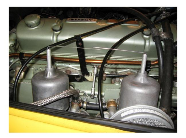
12. With the carburetors synchronized (equal air flow) at 500 rpm, turn the Jet (Mixture) Adjusting Screws (#2) an equal amount (CLOCKWISE for richer, COUNTERCLOCKWISE for leaner) until the fastest idle speed is obtained, consistent with even firing. \*\*
