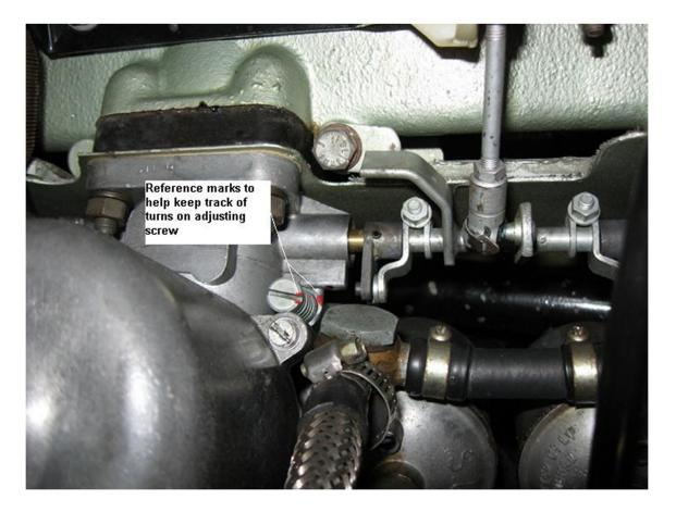
8. Re-install the carburetor pistons. With chokes fully off (carb jet levers as far down as they will go), check to make sure that each piston, when raised, falls smoothly and completely to the bridge
